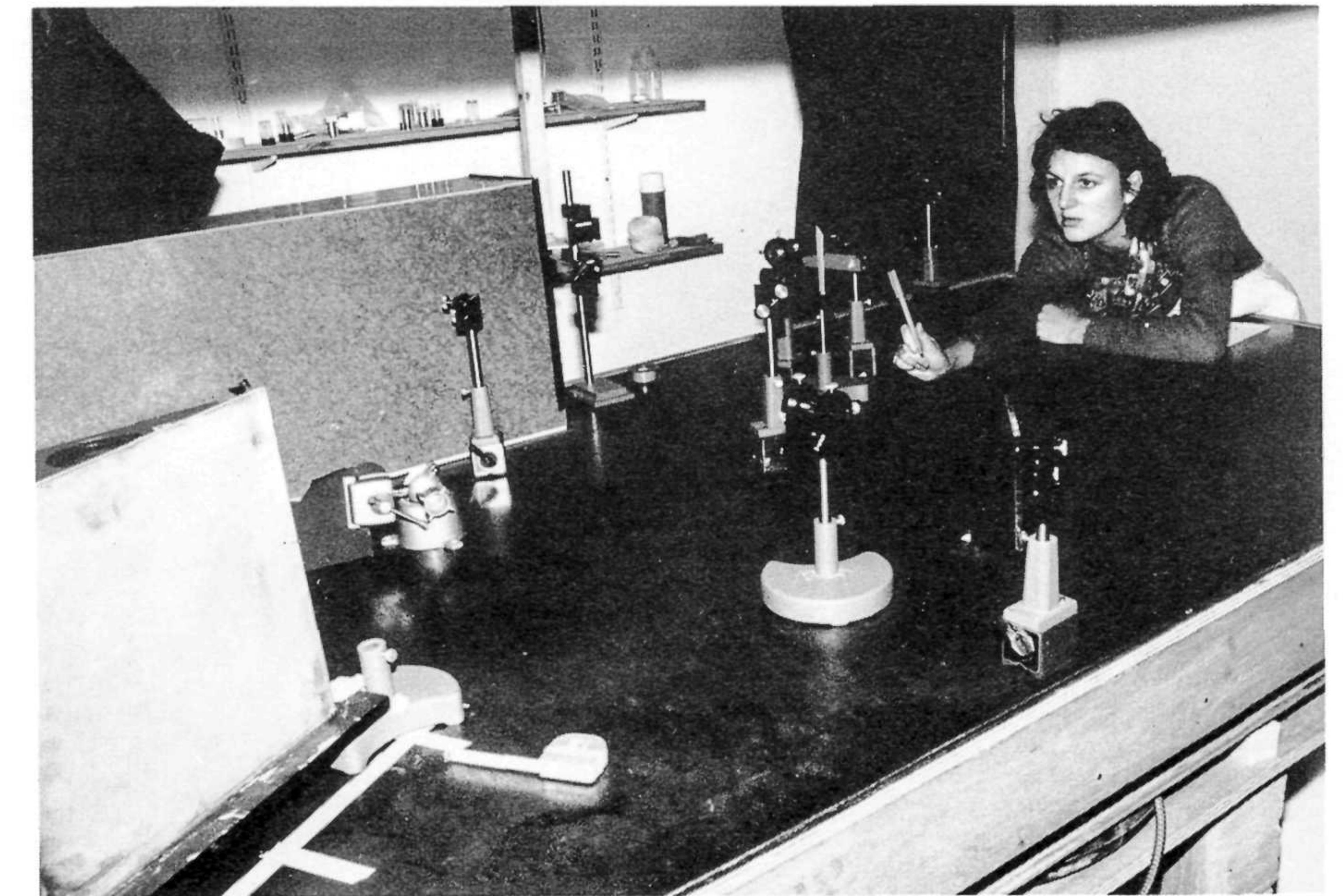
A holographic 'camera' can be very complex; Susan Gamble aligns optical components for the 'Body in Question' series of holograms. The laser is housed in the box in the top left hand corner of the table. The white screen in the bottom left hand corner is a diffuser.
